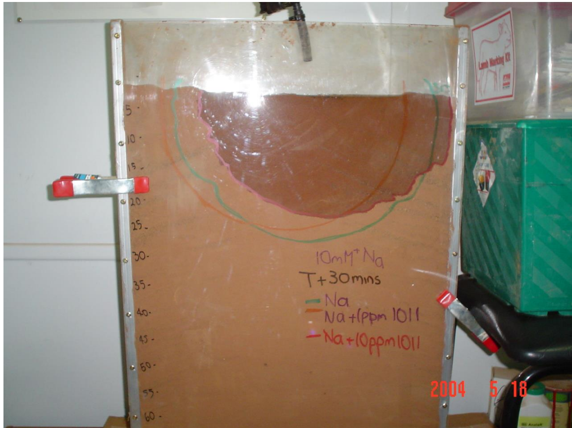
Picture 4: When increased salinity of the irrigation water was used the impact of AG30 in reducing infiltration rates was also reduced. To decrease infiltration rates where saline water is being used would require higher AG30 rates than what would be required in better quality irrigation water.
